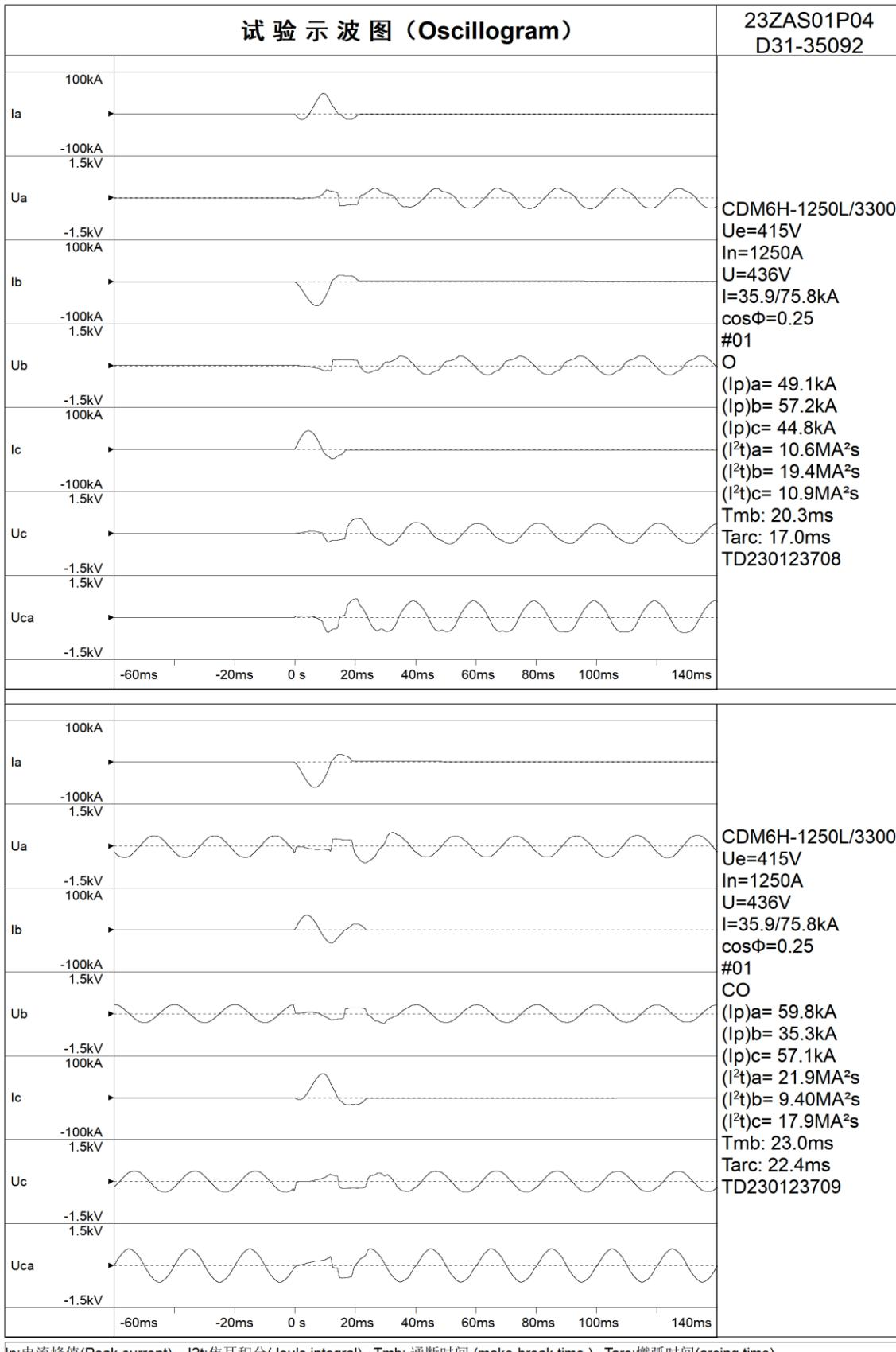
Ip:电流峰值(Peak current) I<sup>2</sup>t:焦耳积分(Joule integral) Tmb: 通断时间 (make-break time ) Tarc:燃弧时间(arcing time)
